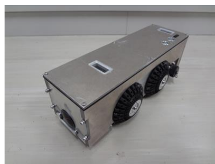
Fig. 1 Autonomous pipe inspection robot
