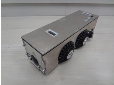
Fig. 2 Autonomous pipe inspection robot.
